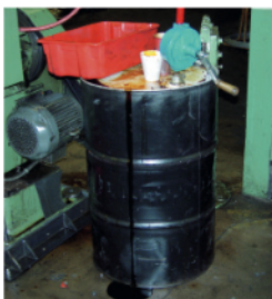
No more pump drips sliding down the side of the drum and onto the floor.
